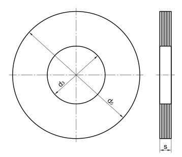
Designation of a wearing washer for wheel- $\emptyset$  d1 = 300 mm,  $axle-\emptyset d3 = 50$  mm, thickness of the washer s = 10 mm:
