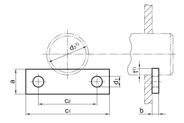
The axle brackets have to be placed in way, that the fastening screws are not stressed by the pressure of the axle.
