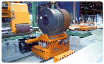
SCISSOR LIFT TABLE, SHOULDERED BY THE ATLAS WHEEL BLOCK SYSTEM Universal, modern, modular and always accurate
